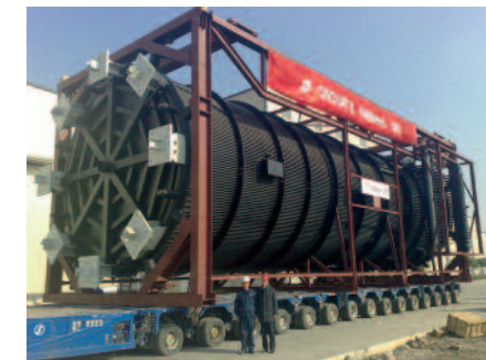
The first of three natural-circulation boilers manufactured at Oschatz Energy & Environment in Nanjing for the world's biggest sulphuric acid plant in Saudi Arabia has now been delivered. The boiler, which weighs more than 300 t, is part of three complete waste heat systems that Oschatz is producing for the plant in Mäaden. The dimensions of the three accompanying boilers puts them among the world's biggest aggregates manufactured in one piece.
